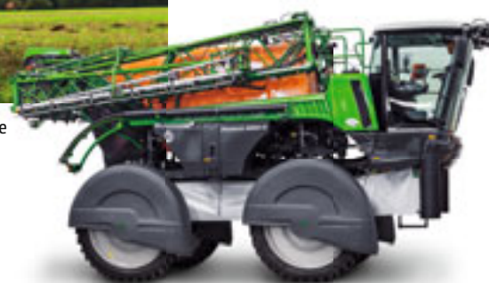
The SunflowerKit for the Pantera-H self-propelled sprayer serves, when spraying or fertilising in tall crops, to prevent both damage to the crop as well as the underside of the machine. It ensures optimum safeguarding of the plants and, at the same time, protects the running gear units of the Pantera-H self propelled sprayer.
