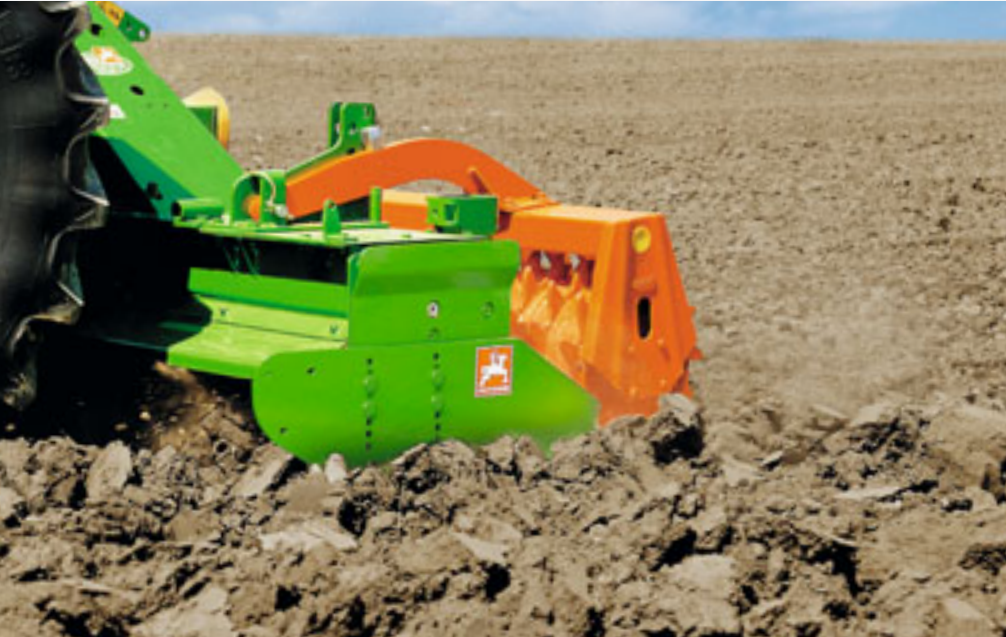
KE rotary harrow with tooth packer roller
