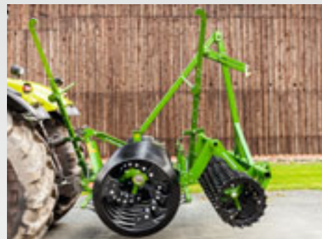
The optional NRP breaker ring roller is available as a following roller to give a more intensive levelling and crumbling effect.
