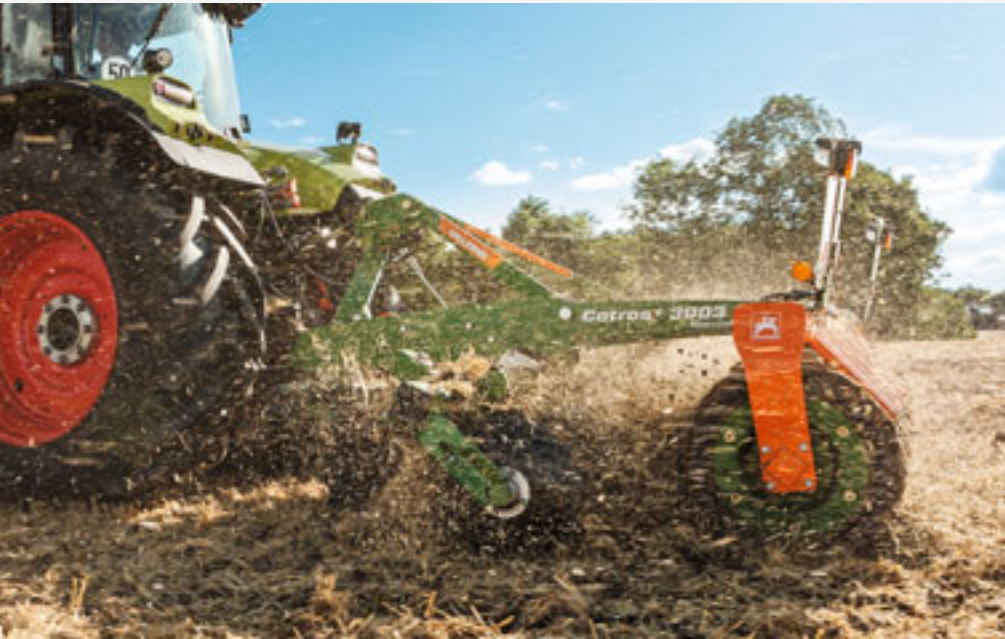
Catros+ 3003 Special with serrated discs in 3 m working width
