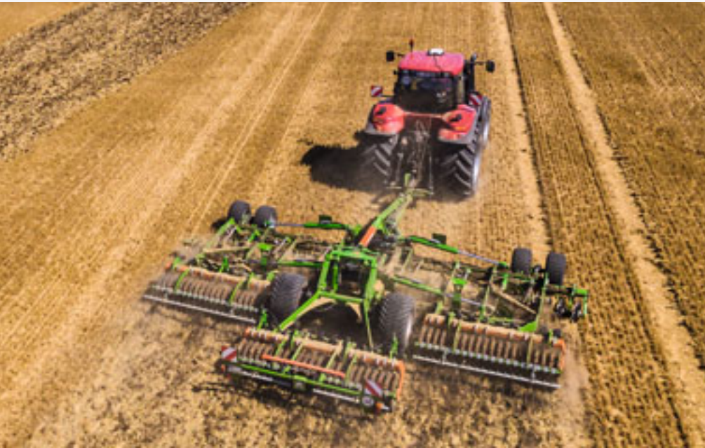
Catros + 8003-2TX with wedge ring roller with Matrix tyre profile in 8 m working width
