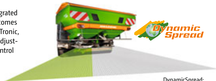
DynamicSpread: 64 or 128 fold part-width section control on the ZA-TS
