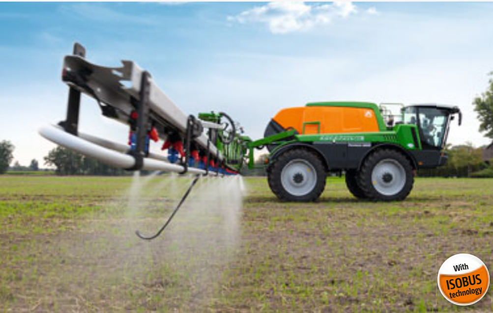
Pantera 4502 self-propelled sprayer with a ground clearance of 1.2 m
