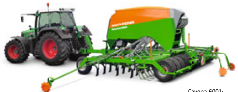
Cayena 6001: 36 tine coultters, 16.6 cm row spacing – forward speeds of up to 15 km/h
