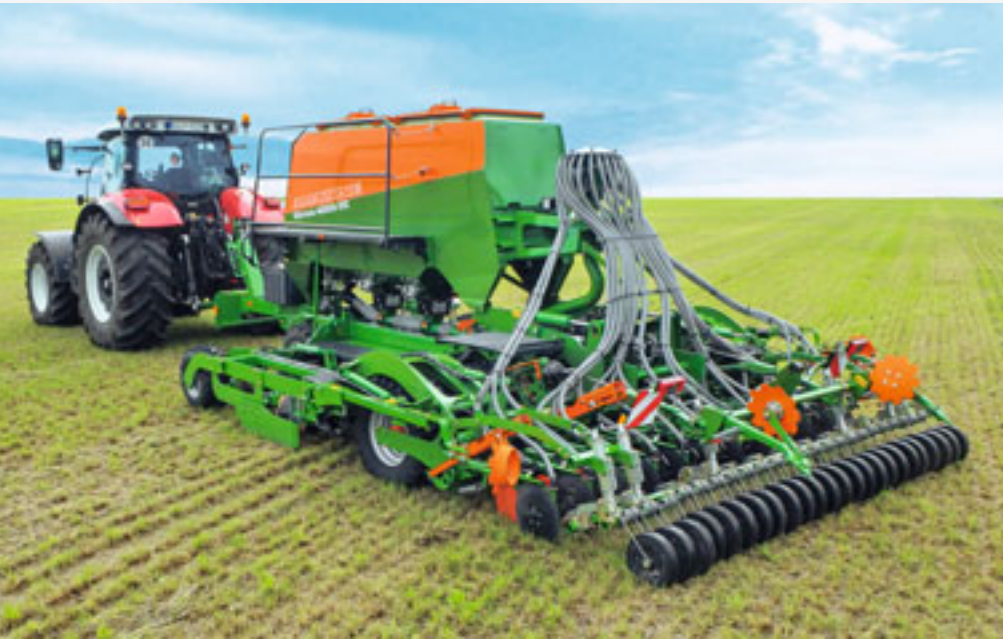
Cirrus 4003-2C with RoTeC pro single disc coulters and 4000 litre pressurised tank for seed and fertiliser
