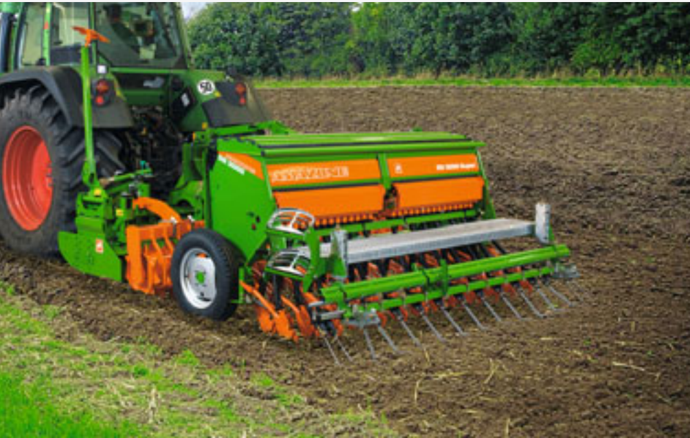
D9 3000 Super with Exact following harrow in combination with rotary harrow and tooth packer roller
