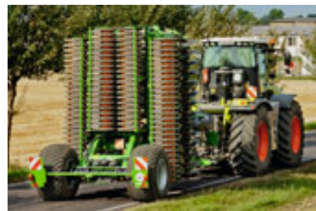
Safe road transport with a transport width of less than 3 m is assured by the main frame which is hydraulically folding as standard.
