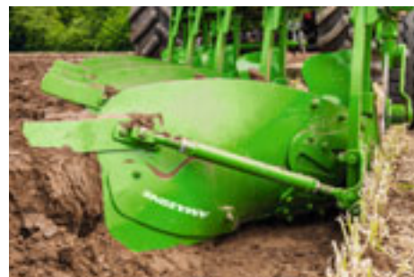
The X-blade widening share is a specific mouldboard extension mounted on the last plough body and creates, on average, a 30% wider furrow bottom.
