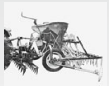
1967 First modern sowing combination with reciprocating power harrow
