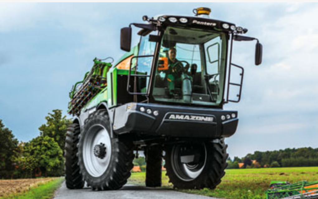
Pantera 4502 self-propelled sprayer is compact in design and comes with four wheel drive
