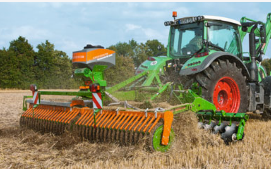
Catros + 5002-2 in 5 m working width with serrated discs (510 mm diameter)
