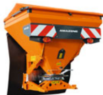
The E+S Hydro 751 winter salt spreader is equipped with a 750 litre hopper, hydraulic spreading disc drive and a forward speed related spread rate regulation
