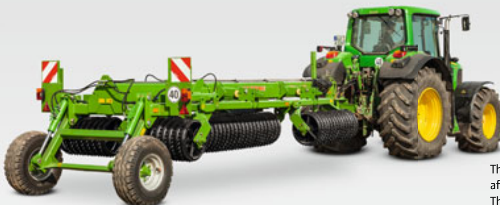
AW 9400 in transport – also 40 km/h is permissible
