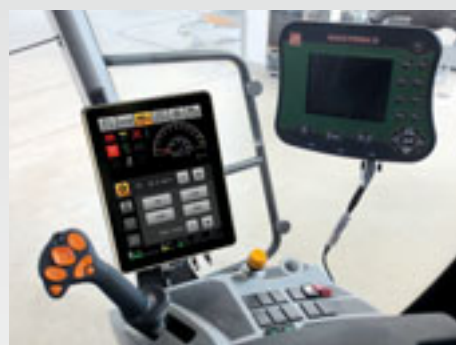
Via the AmaPilot multi-function joystick and the AMADRIVE operator terminal, the Pantera offers a comfortable and simple operation.
