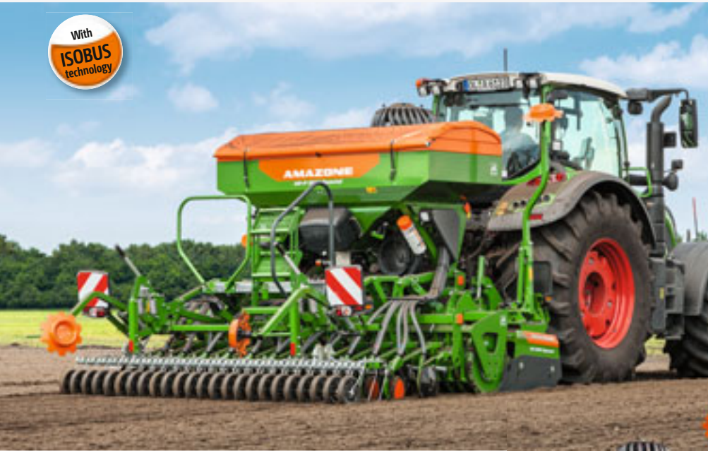
AD-P 3001 Special RoTeC coulters and roller harrow
