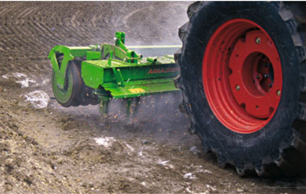
Extreme stone test track: The tine spring fixing on the rotary harrow and cultivator allows the tines to give way when stones are encountered.
