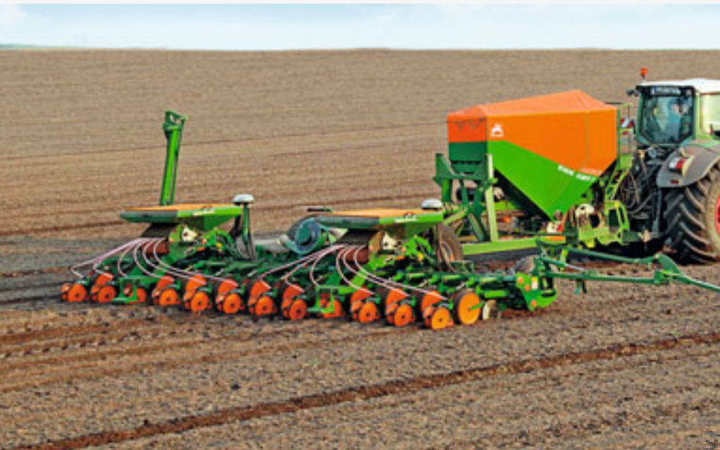
EDX 9000-TC trailed precision air seeder, 9 m working width
